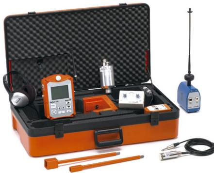
This robust plastic case offers space for all system components. The Receiver and two transmitters can be charged simultaneously inside the closed case.
