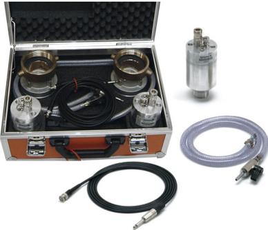
Hydrophones do not pick up the sound from the pipe material, but directly out of the water column. This offers a considerable improvement of the location range, especially with correlations on plastic pipes. Correlating leaks over 1500 ft. is possible.
