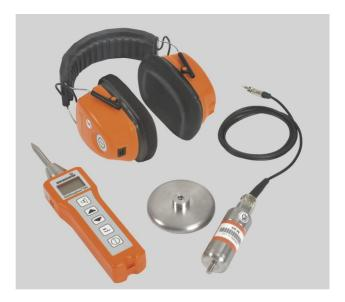
certain noises such as the deep-pitched sounds typical from leaks in plastic pipes and higher frequencies from metallic pipes.
